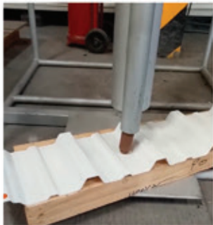
BULLET IMPACT TEST (0.755kg)
