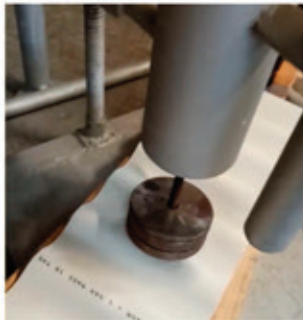
BALL IMPACT TEST (2.495kg)
